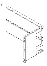
Place 2nd panel below the top panel. Use (2) M4 screws to secure 2nd panel.
