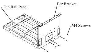
1 Place panel on flat surface. Place ear bracket next to din rail panel. Align (4) M4 screws with screw holes on right side of panel as illustration above.
