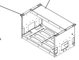
Place Solid panel as show in the illustration above. Align mounting holes on right side panel with front panel mounting holes. Secure ear bracket to solid panel with (2) M4 screws. Follow the same process with left hand side for installing mounting screws..
