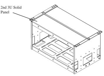
4 Place 2nd 3U solid panel as show in the illustration above. Following step 3 for installation mounting screws for right and left hand side.
