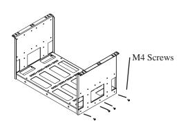
**2** Repeat Step 1 for left hand side ear bracket . Secure (4) M4 screws.
