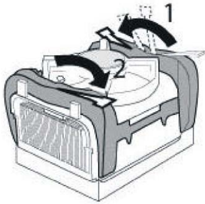
Figure 3-9a: Installing the Fan Heatsink (4) Close Clip Levers, One at a Time
