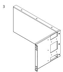
Use (3) M4 screw to mount ear bracket to panel
