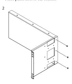
Align mounting holes on the panel with mounting holes on the ear bracket.
